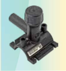
MULTISEAL TAPPING TEE STACKLOAD PE100 Water PN16 / Gas 10 Bar (UK Gas Applications - Gas 5.5 Bar (Class B) / Gas 7 Bar (Class C)) 20-32mm Outlet d63x20-355x32
