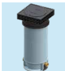
AVK PENTOBX WATER METER BOUNDARY BOX, CONTAMINATED GROUND GRADE B VERSION, SEALED SERIES 8054/52-002 BS 5834-1:2017 PN16 Polypropylene frame ¾" BSP
