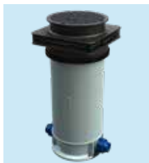
AVK PENTOBX WATER METER BOUNDARY BOX GRADE B VERSION, SEALED SERIES 8054/2211 BS 5834-1:2017 PN16 Polypropylene frame d20-32, ¼" BSP, ½" HG
