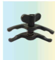
ELBOW CLAMPS For alignment and restraint of pipe and electrofusion fittings 20, 25 and 32mm
