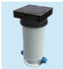
AVK PENTOBX WATER METER BOUNDARY BOX GRADE B VERSION, SEALED SERIES 8054/5211 BS 5834-1:2017 PN16 Polypropylene frame d20-32, ¼" BSP, ½" HG
