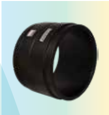
LARGE DIAMETER COUPLER PE100 SDR 11-26 - Water PN16 / Gas 10 Bar SDR 17-26 - Water PN10 / Gas 6 Bar d450 - 630
